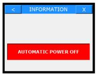
The machine gives a warning before the power is actually switched off. The power-off can be canceled by pressing anywhere at the screen, or by pressing any button at the remote control.
