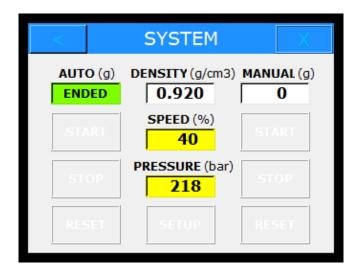
When the AUTO grease counter reaches zero, the pump stops, and the AUTO grease counter turns green, and flashes "ENDED".
