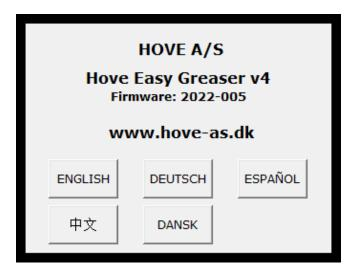
The MAIN screen appears in the display a few seconds after switching on the Hove Easy Grease. Select the required language by pressing the corresponding button on the screen.
