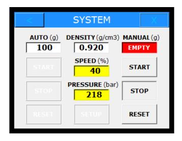
If the built-in flowmeter does not register the expected grease flow for a predetermined amount of time, either during manual or automatic dosing, the pump stops, and the grease counter turns red and flashes "EMPTY".
