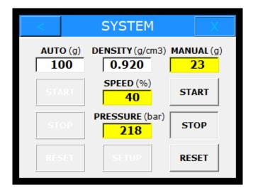
When the MANUAL grease counter reaches the required amount or if you want to pause the pumping, press the MANUAL STOP button.
