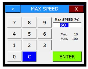
Enter the pump speed limit (% of max).
