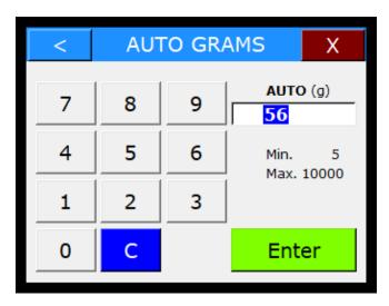
Enter the required grease dose. The entered value must be within the "Min." and "Max." limits. Otherwise, the setting will not be altered.
