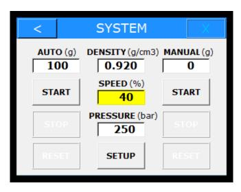
After a few seconds the AUTO grease counter changes to the set value and the machine is ready again.
