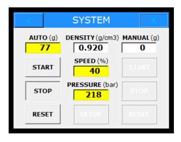
If desired, you can pause the pump during the automatic dosing by pressing the AUTO STOP button.
