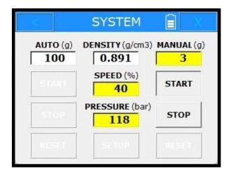
The pump starts, and the dosed amount of grease counts from zero and upwards in the MANUAL (g) field.
