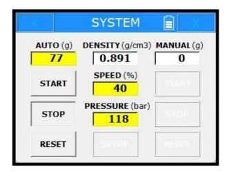
Press **START** to continue AUTOMATIC DOSING or press **RESET** to end it.
