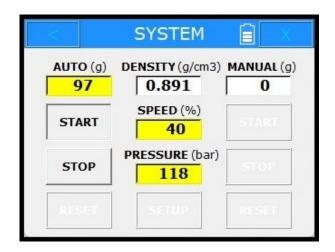
The pump starts, and the **remaining** amount of grease to be dosed is counted down in the AUTO (g) field.
