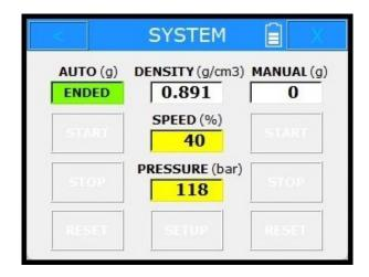
When the AUTO grease counter reaches zero, the pump stops, and the AUTO grease counter turns green, and flashes "ENDED". After a few seconds the AUTO grease counter changes to the set value and the machine is ready again.
