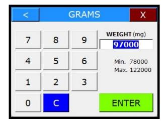
Input the noted weight in mg, e.g., 97g = 97000. Dispense 100g again and check that the weight is 100g +/- 3g; otherwise repeat the calibration steps max. 3 times.
