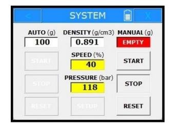
Press **START** to continue MANUAL DOSING or press **RESET** to end it
