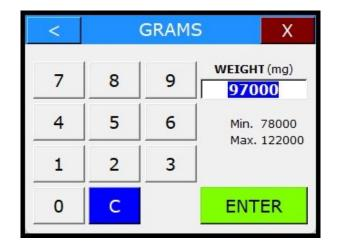
Input the noted weight in mg, e.g., 97g = 97000. Dispense 100g again and check that the weight is 100g +/-3g; otherwise repeat the calibration steps max. 3 times.
