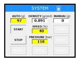
The pump starts, and the **remaining** amount of grease to be dosed is counted down in the AUTO (g) field.
