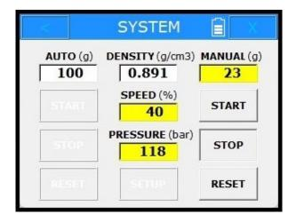
When the MANUAL grease counter reaches the desired amount, press **STOP** and then **RESET**.
