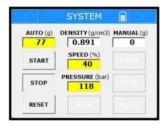
Press **START** to continue AUTOMATIC DOSING or press **RESET** to end it.
