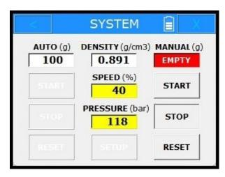
Press **START** to continue MANUAL DOSING or press **RESET** to end it
