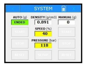
When the AUTO grease counter reaches zero, the pump stops, and the AUTO grease counter turns green, and flashes "ENDED". After a few seconds the AUTO grease counter changes to the set value and the machine is ready again.
