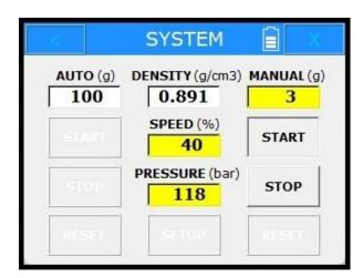
The pump starts, and the dosed amount of grease counts from zero and upwards in the MANUAL (g) field.
