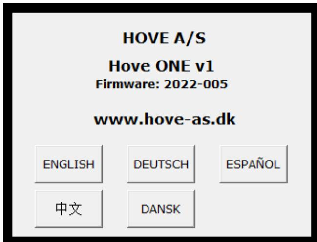
The MAIN screen appears in the display a few seconds after switching on the Hove ONE. Select the required language by pressing the corresponding button on the screen.
